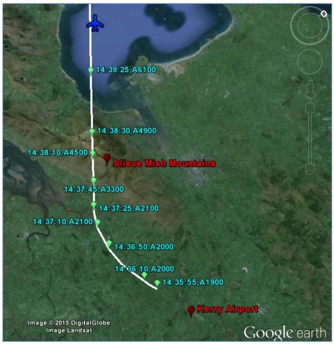
**Note**: The labels comprise a UTC timestamp and the aircraft altitude in feet, based on the airfield pressure on the day (1024 hPa)
